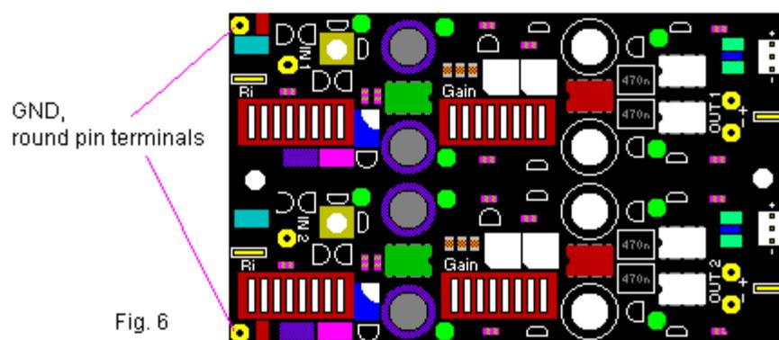
**GND.** The two round GND pin terminals must be connected with short wires to the solder tags on the attached Screen Plate P117-02. This is normally done by the manufacturer before shipping. Please observe that no conductor tracks on the PC board unintendedly connect to the Screen Plate or other external circuits. See fig. 6. (See also [MOUNTING](#)).
