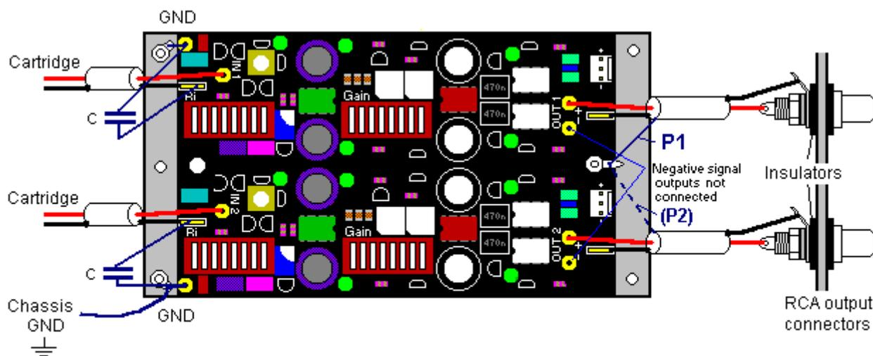
Fig.10. Mounting CT100 into a non-metal enclosure/turntable.
