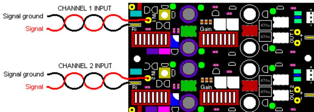
Fig. 5. Connecting the cartridge using unscreened wires.
