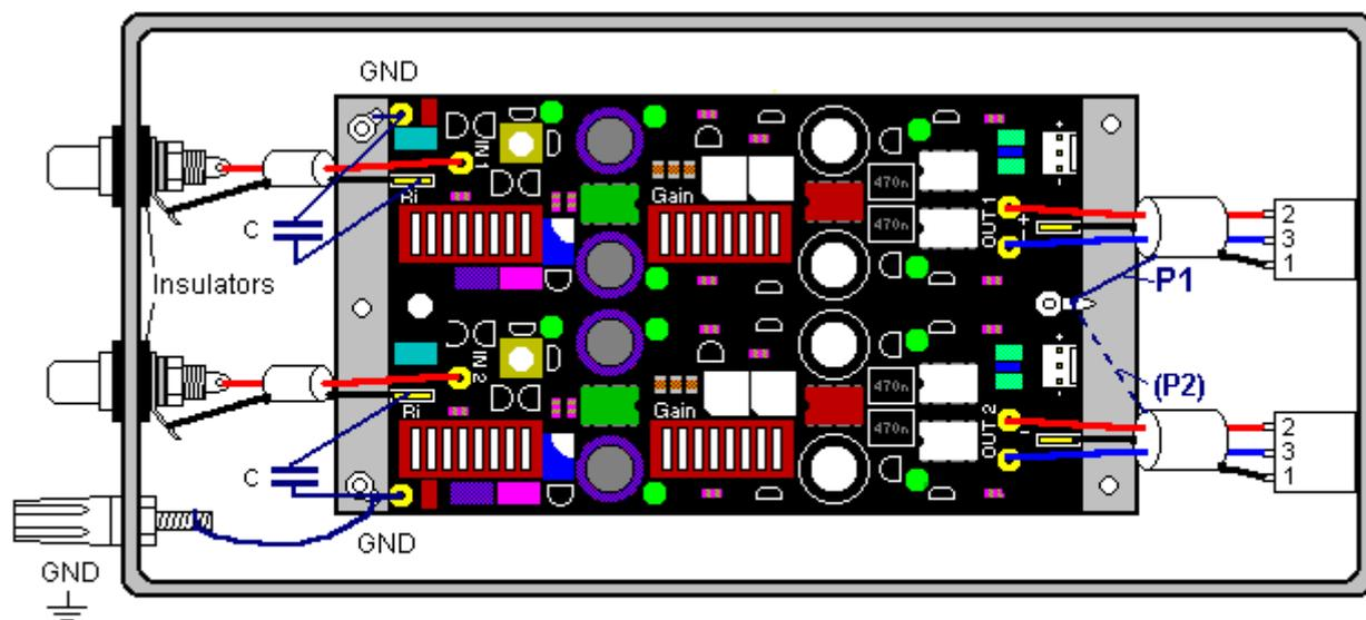
Fig.11. Mounting CT100 into a screened metal enclosure.
