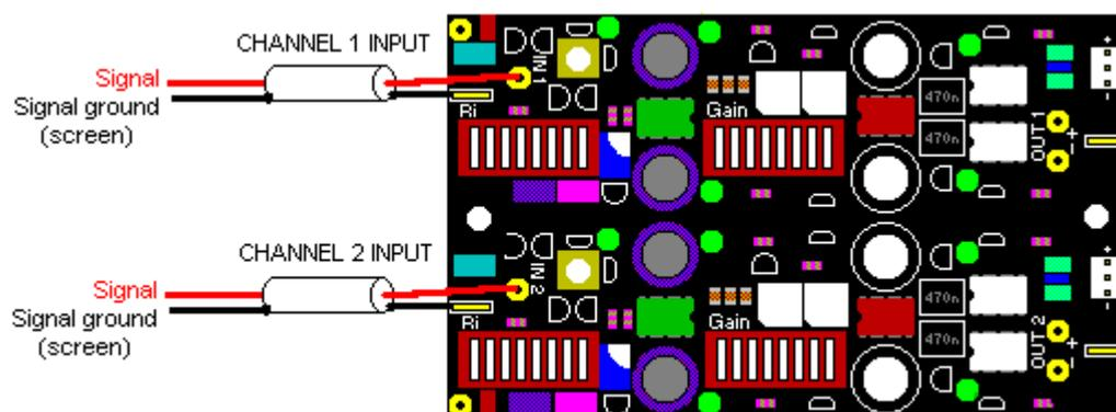
Fig. 4. Connecting the cartridge using screened cables.
